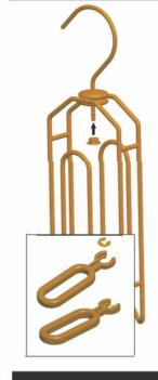
Fit washer over groove until it clicks into place using tool as shown in diagram.
